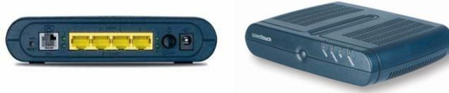
To configure your speedtouch router, you must first reset it. At the back of the router on the far left you will see a small hole where a pen/pin or similar object can be pushed in to reset the router. You will need to hold the object on the reset button for one minute, whilst the router is powered on.
